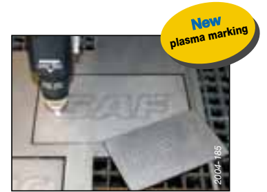
thickness 3 mm - Argon - 12 A speed 2.5 m/min.
